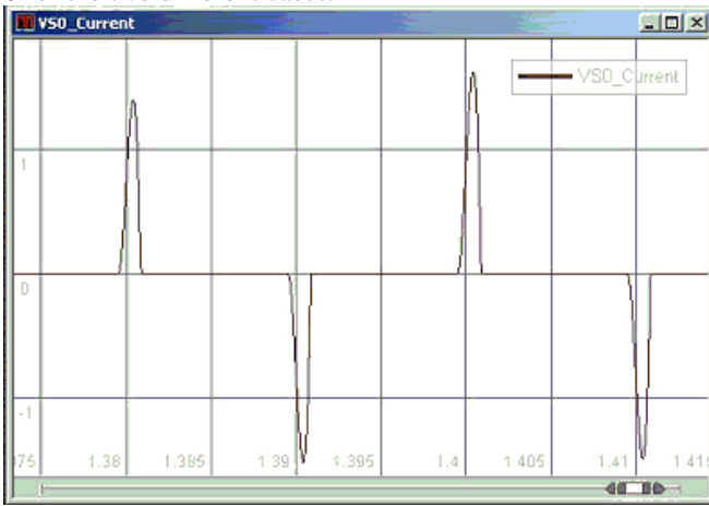
Fig. 10 - Source current under no-load conditions (x-axis in [s] and y-axis in [A]).
