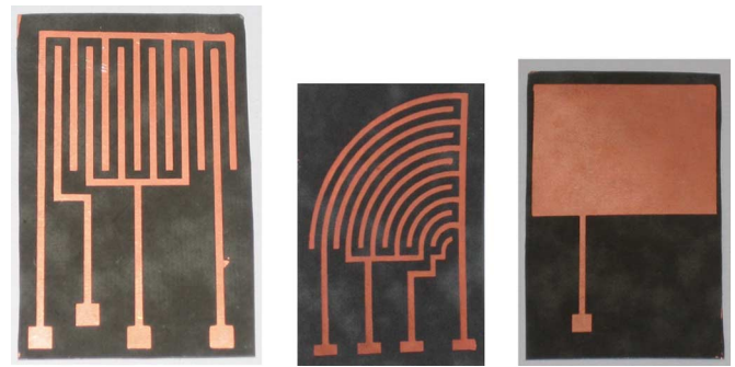
Fig. 8. Photographs of the (a) meander sensor, (b) quarter-circular sensor, and (c) sensor backplane.
