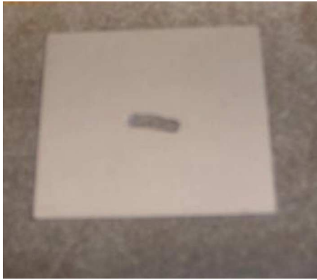
Fig. 9. Sample 1.5-mm-thick damaged Duroid 6010.
