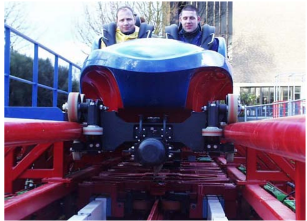
Fig. 21. Linear PM coaster launcher at Six Flags Holland. (Photograph by kind permission, KumBak Coasters)
